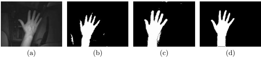
Fig. 5. Cues for hand segmentation: The grabbed image (a), when only thresholded (b) or background subtracted (c). Combination of background subtraction and thresholding (d)
