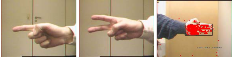
Fig. 2. Examples of static hand gestures and, in the right picture, the result of hand segmentation for hand tracking.
