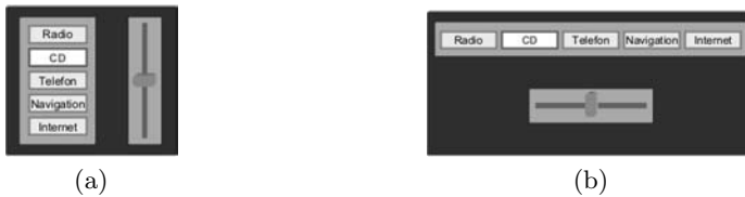
Fig. 3. Vertical (a) and horizontal alignment (b) of menu points with visual presentation for indirect (left) and direct (right) manipulation
