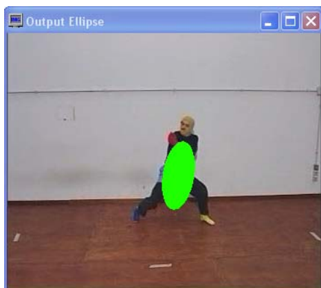
Fig. 2. Silhouette shape and orientation. The ellipse approximates the silhouette; its axes give an approximation of the silhouette's orientation.
