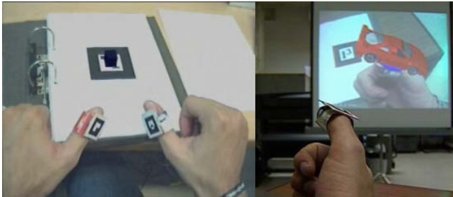
Fig. 4. (Left) Manipulating Magic Rings , a new type of Tangible Interface, within the context of a Magic Book . (Right) Picking an object with the finger using a Magic Ring .
