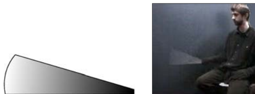
Fig. 3. Note how a moving baton appears as a wedge with an intensity gradient in the camera frame (right) giving the general form illustrated with an artificial border (left).
