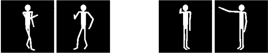
Fig. 1. Two postures of the stick figure (each rendered from two different points of view). Such images are compared to segmented input images to identify the posture of the input figure. Obviously it is helpful to have at least two views of a scene to disambiguate (self-)occlusions.
